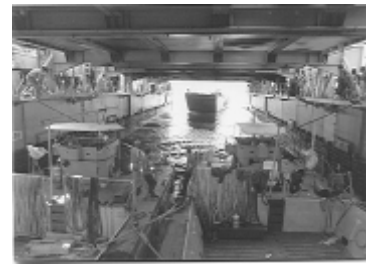
The rear door of the ship opens and the amphibious vessel floats out.
